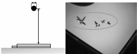
图 3 低温气泡测试方法和现象 Fig.3 Test method and appearance of cold bubble
