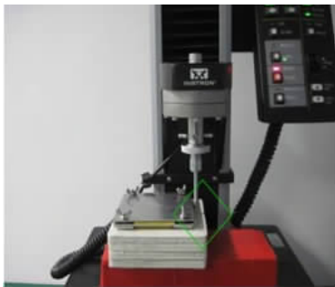
图 1 Push Mura 测试设备 Fig.1 Test instrument of Push Mura
